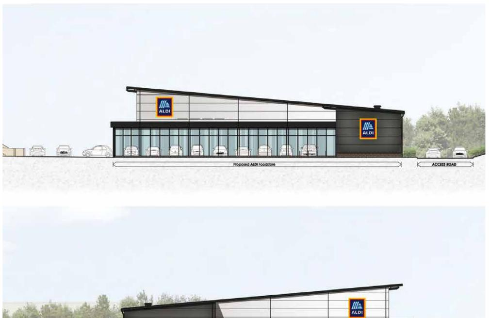
high-level ribbon windows to the southern elevation, together with a contemporary pressed metal feature canopy assist in creating and active facade.
